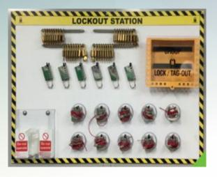
As such, applying LOTOTO (Lock-Out – Tag-Out – Try-Out) which is a safety procedure for isolating equipment to ensure maintenance and cleaning can be undertaken safely has the potential to significantly reduce risks and improve the safety of workers.
