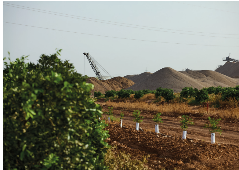
Progressive restoration and revegetation measures at an aggregate extraction site to promote ecological recovery and landscape integration. [15]
