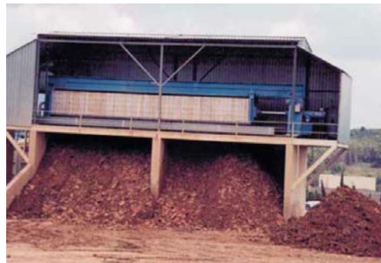
Thickening tank and press filter – Sand and gravel pit – Terrassa site – Haymsa – Spain
