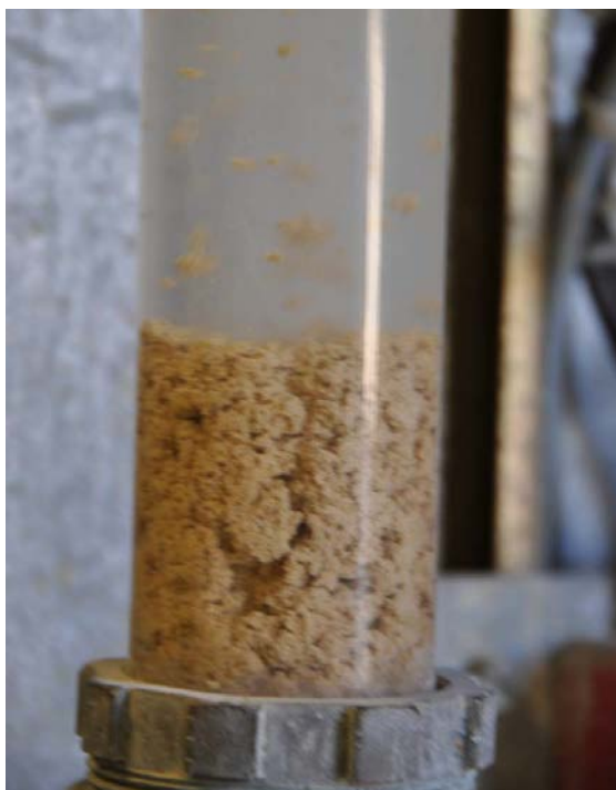
End of water control cycle by flocculant, causing the sludge to flocculate and settle at the bottom
