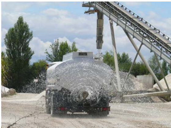
Water spray in tracks for dust prevention – UNICEM
