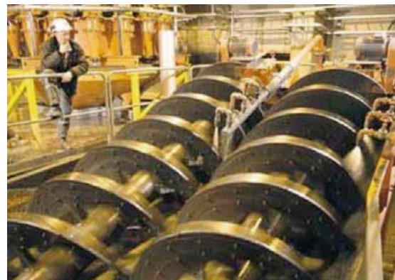
Spiral classifier – Seldom used in the aggregates industry.
