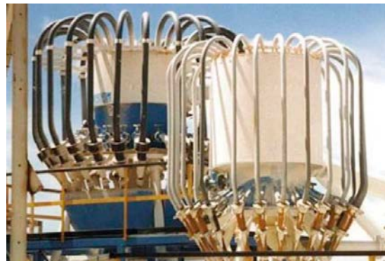
Hydro cyclones – Fines and ultra fines recovery – Readily replaceable modules
