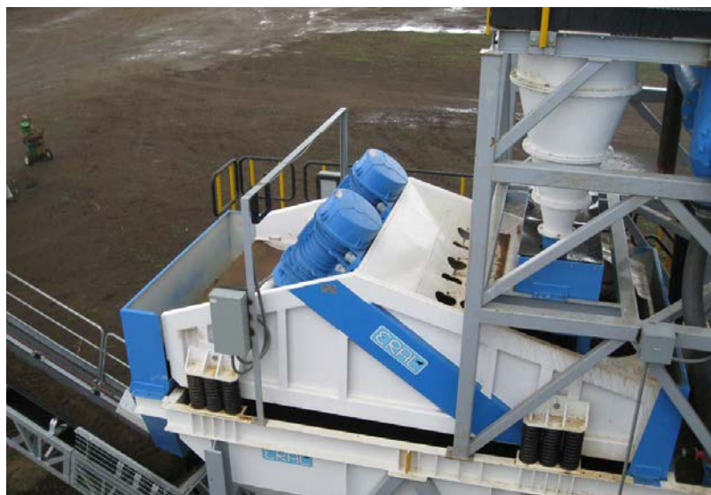
Diverse models of high frequency screens for precise sorting process
