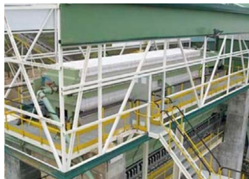
Filter press - Dewatering sludge and wastewater recovery process
