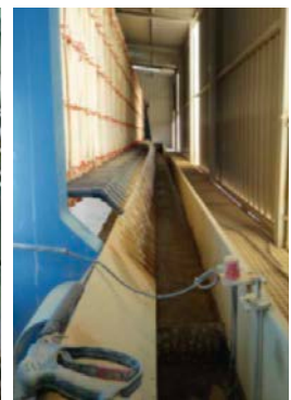
Filter press - Dewatering sludge and wastewater recovery process
