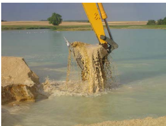
Aggregates extraction under water table – UNICEM
