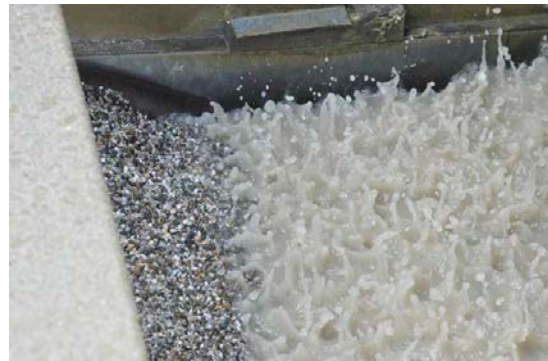
Dewatering screen – Gravel dewatering and filtration of fine materials - Montpouillan - France
